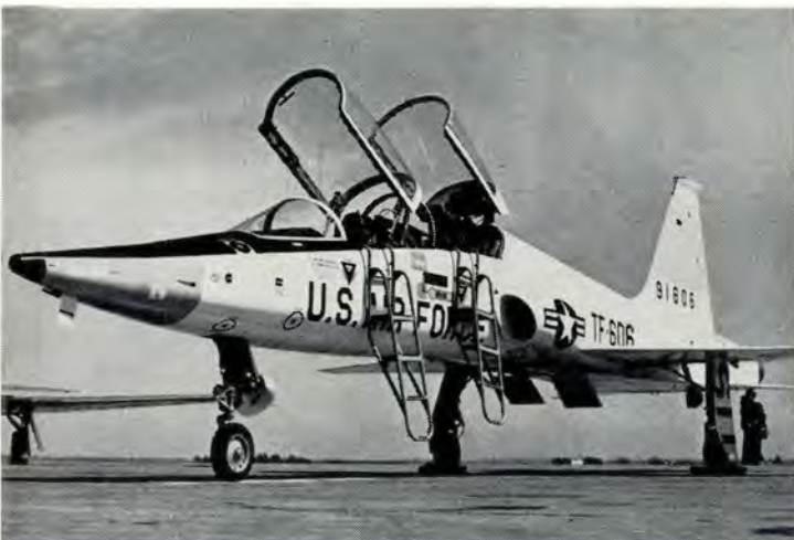
Talon, Air Force's new jet trainer, features twin engine reliability, supersonic speed, fine visibility. Photos show panel, twin canopies, liquid oxygen refill from ground level, excellent, non-obstructed view from cockpit. In picture above, T-38 is welcomed to ATC at Randolph AFB. Photos of exterior view of T-38 showing twin canopies and dual tailpipes, courtesy of Mr. Les Bland.
