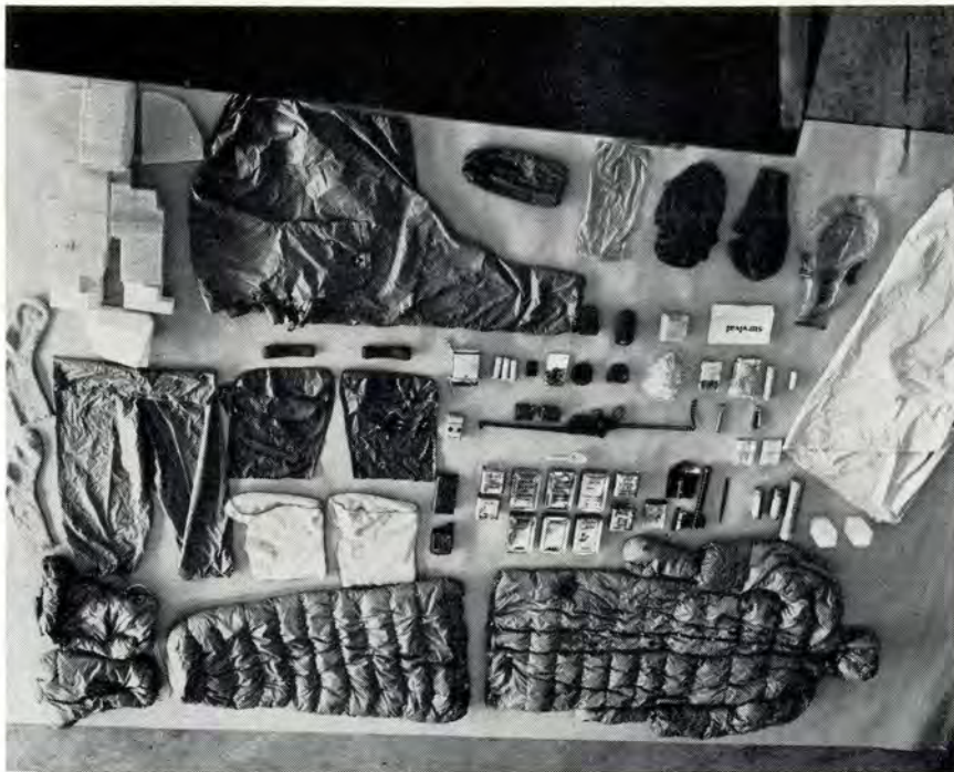
Survival gear in B-58 escape capsule is vacuum packed and designed to protect downed airman on land and sea. During tests men have lived in relative comfort in capsule for three days.
